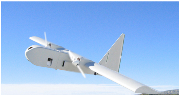
Figure 36: Students in the FrankenEye program used the DragonEye aircraft shown above as a basis for design. Students modified and reassembled DragonEye UAS, including newly designed pieces. The DragonEye has proven a useful and robust UAS platform for dangerous environments such as volcanoes and fires.
