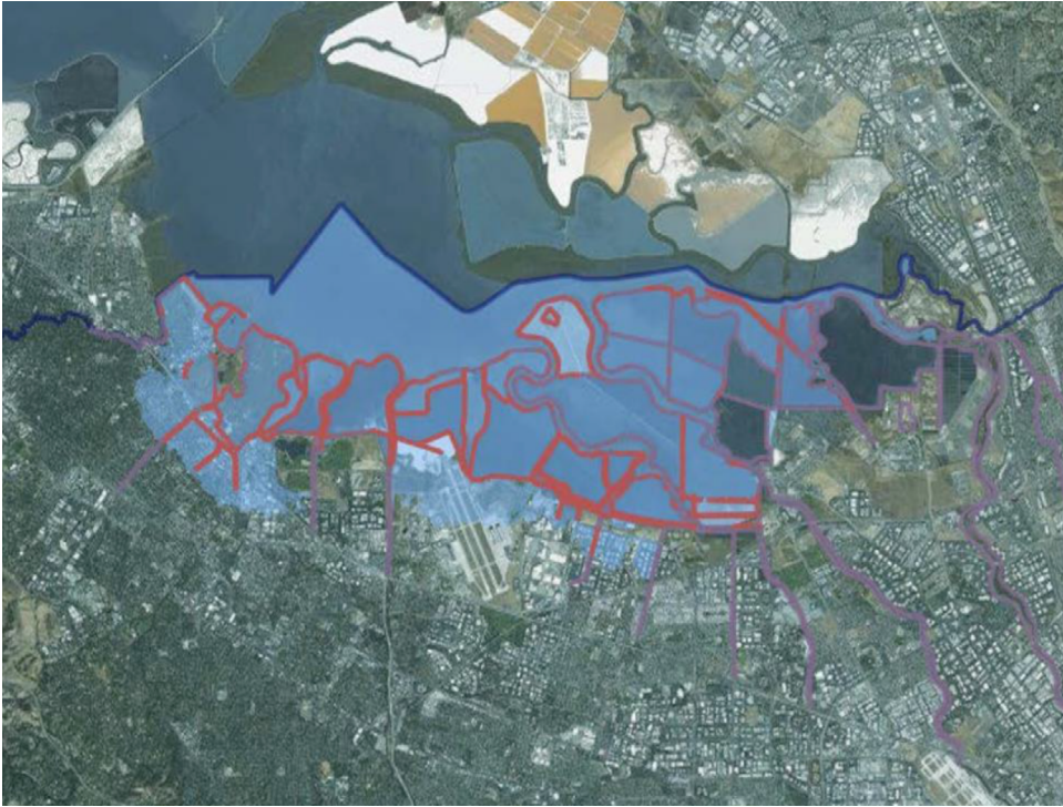
Figure 19: Projected high tide water levels in south San Francisco Bay with a 50cm rise in global mean sea level rise. The NASA-ARC facility can be identified by the airfield (2 runways oriented vertically) located just left of center.
