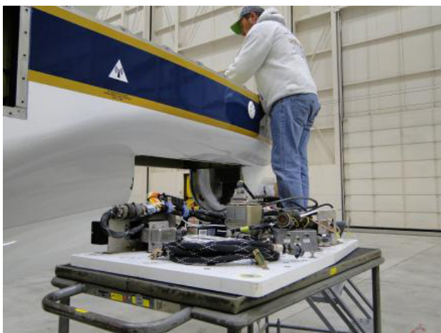
Figure 29: An MMS payload is installed on the DC-8.
