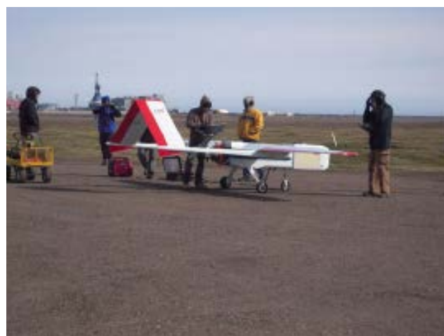
Figure 23: Pre-flight checks are completed on the SIERRA aircraft, one of several UAS managed by the Airborne Science Advanced Planning team.
