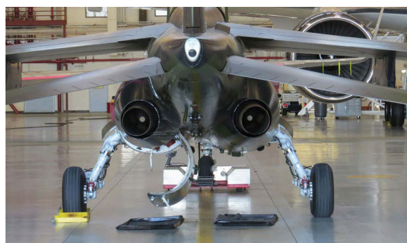
Figure 8: A view of the Alpha Jet research platform, based at NASA-ARC. Instruments are housed in specially designed wing pods.
