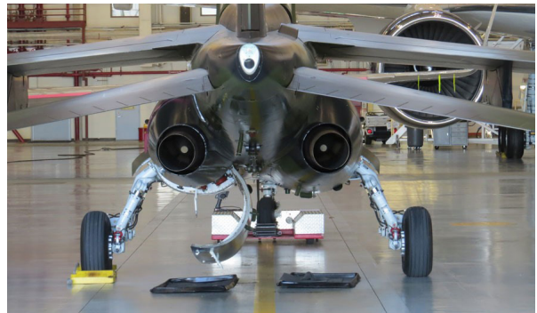
Figure 6: A view of the Alpha Jet research platform, based at NASA-ARC. Instruments are housed in specially designed wing pods.
