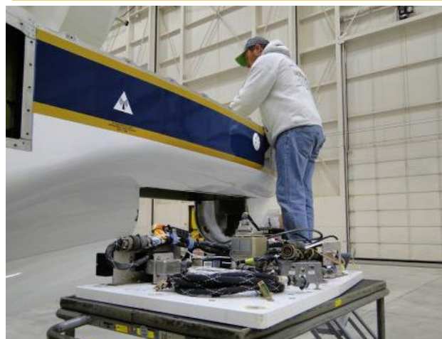
Figure 23: An MMS payload is installed on the DC-8.
