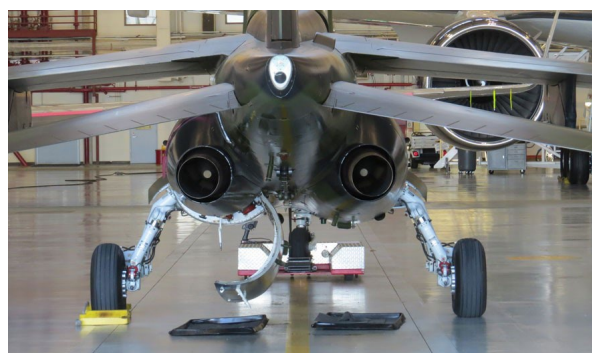
Figure 3: A view of the Alpha Jet research platform, based at NASA-ARC. Instruments are housed in specially designed wing pods.
