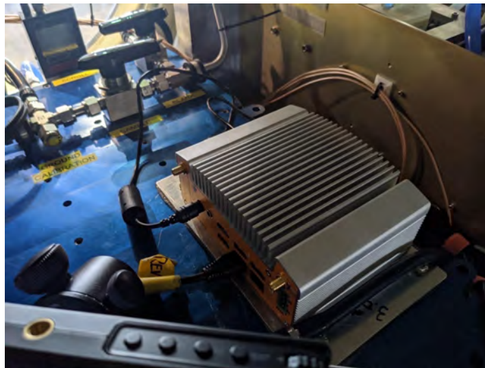
Inmarsat Router/Display system on the LaRC HU-25 Aircraft in support of ACTIVATE
