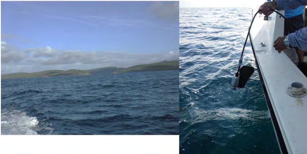
Left: Entrance of Guánica Bay in southwest Puerto Rico; Right: drop-off camera for video transects collection
