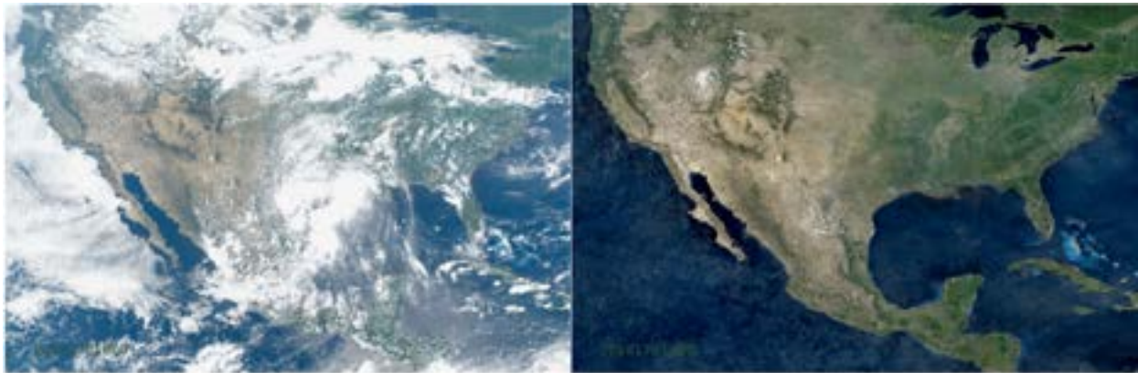
Figure 3: Example of GeoNEX L1G (TOA) and L2G (Surface) BRDF-enhanced reflectance with data from GOES-16/ABI collected over CONUS on 2018/06/18, 19:00UTC.
